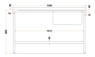
This fully welded 1500mm wide sink from Holmes features a left side drainer with right side bowl and is made from high grade 304 stainless steel. This material is ideal for commercial kitchens as it is strong, smooth and easy to clean as well as highly resistant to corrosion and staining. The sink allows you to create practical and hygienic washing areas in your kitchens, and features a strong undershelf for additional storage.
